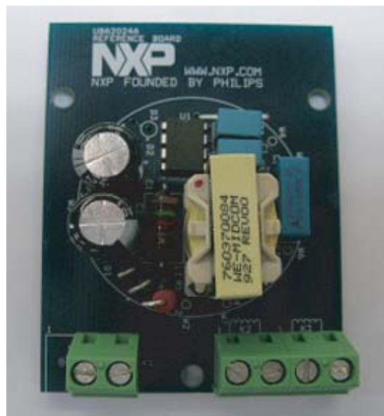
Fig 4. UBA2024AP 120 V (AC) mains demo board
