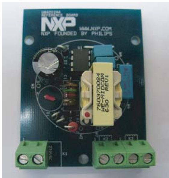
Fig 3. UBA2024AP 230 V (AC) mains demo board
